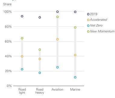
The role of oil in transport falls in all three scenarios. In road transport, this decline largely reflects a combination of improving vehicle efficiency and increasing electrification. In aviation and marine, the decline in oil is driven by the increasing use of bio- and hydrogenderived fuels.
