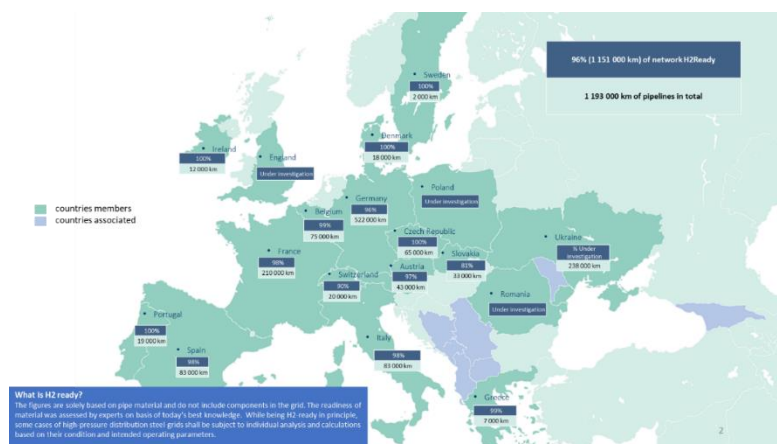
Figure 30: Readiness for pipeline’s repurposing potential. Source: Ready4H2 146 .
