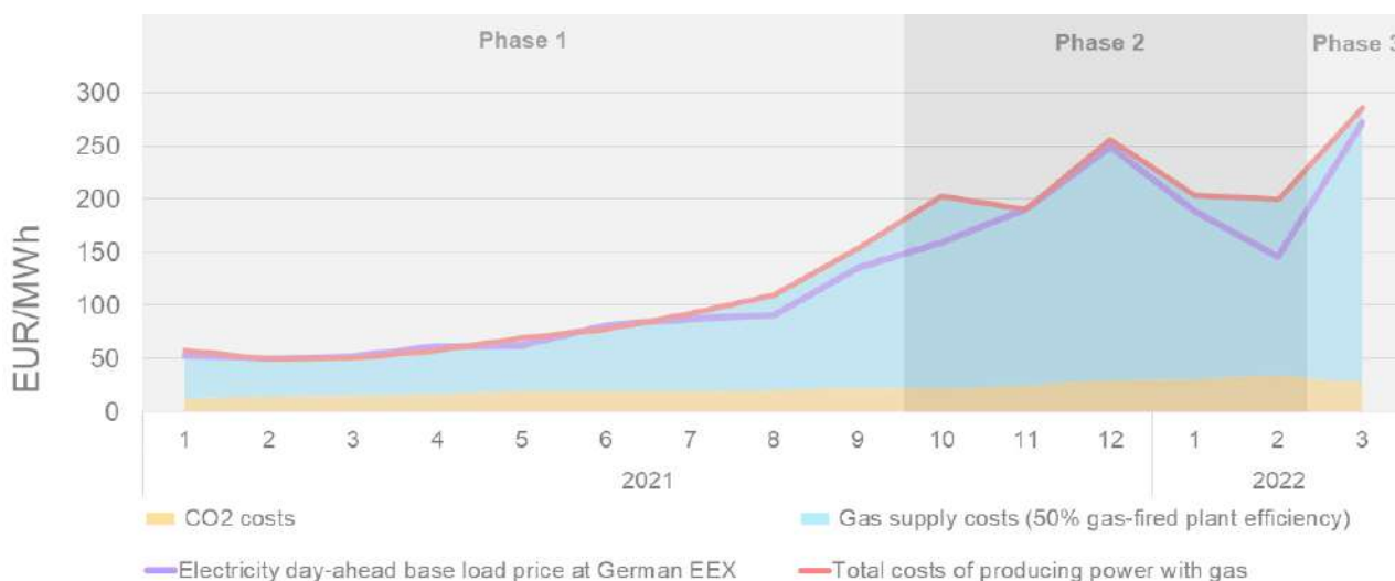
Figure 4: Electricity price development in Germany and breakdown of the costs (EUR/MWh) of producing electricity from gas (May 2021 - March 2022)
